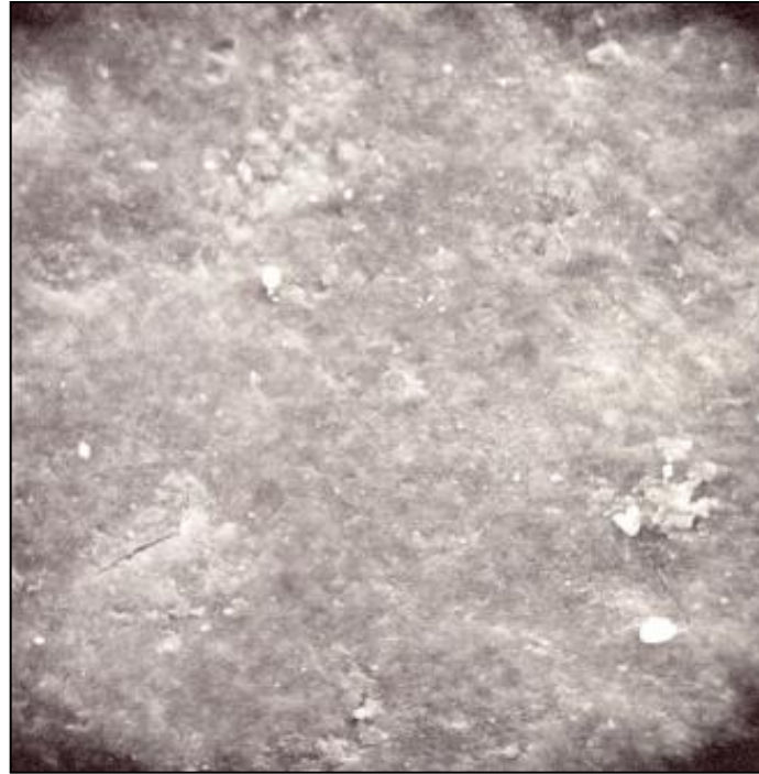
Untreated concrete specimen at 552× magnification
