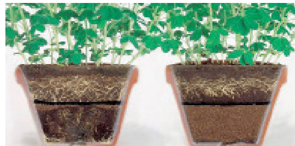
Bituminous Waterproofing without and with antiroot additive Preventol B5.
