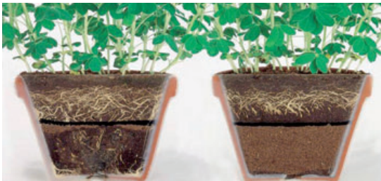
Bituminous Waterproofing membrane without and with antiroot additive Preventol B2 .
